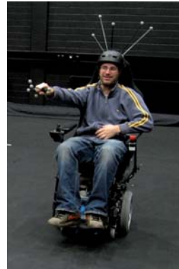
Figure 4 (left). A subject on the robotic wheelchair. The reflective markers for head and hand tracking can be seen.
